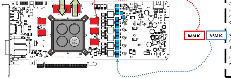
All chips, marked **RED** and **BLUE**, must be passively cooled. This is an example shown on GTX 1080 reference design graphics card. EK suggests users to check their factory cooling solution and locate the ICs which are being actively cooled besides the GPU itself. We recommend applying selfadhesive heat-sinks on the same IC.
