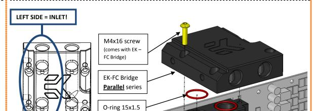
**Type B:** Using EK-FB Bridge Parallel series interconnect for connecting two or more water blocks.
