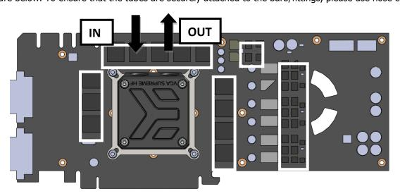
All encircled chips must be passively cooled. This is only an example shown on GTX 480 reference design card. EK suggest you check stock cooler and find out which chips are being cooled by it and place heat sinks on same spaces that are being left exposed. Only this way you will provide some heat transfer from chips, thus optimizing performance of your system.
