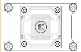
P1 in - P2 or P3 out P2 in - P1 or P4 out P3 in - P4 or P1 out P4 in - P3 or P2 out
