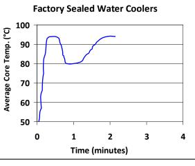
Intel multi-core CPUs have built-in protection (Adaptive Thermal Monitor) that prevents the CPU from exceeding maximum core temperatures, thereby preventing damage to the CPU.
