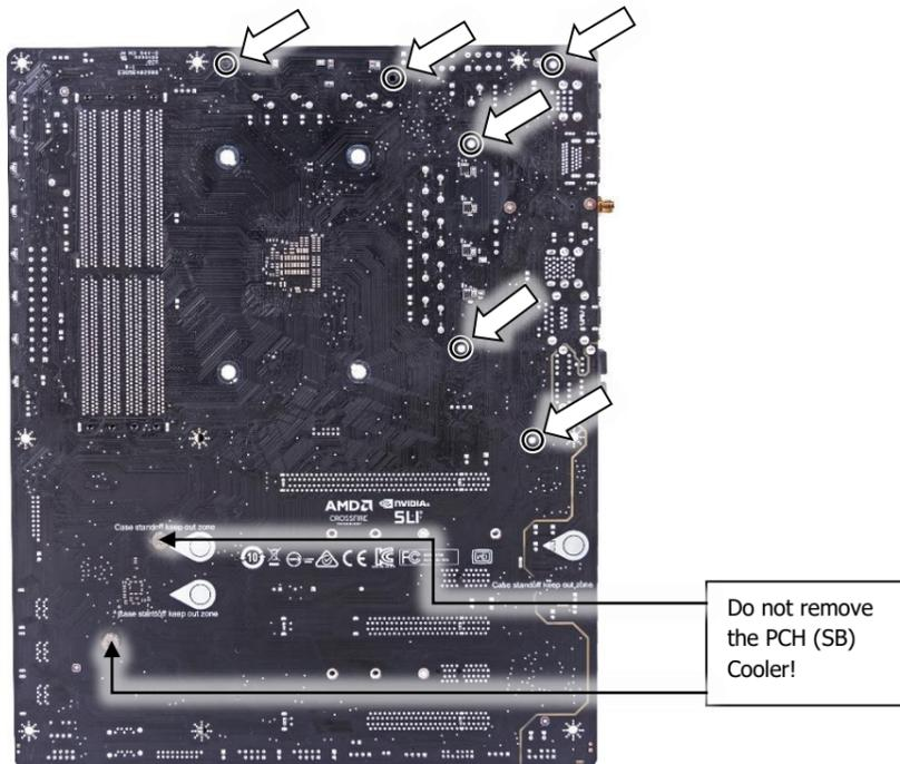
Removing of the original plastic hold-down clamps and the factory backplate: Using Philips-head screwdriver remove the four UNC 6-32 screws securing the original plastic hold-down clamps around the socket as shown on the sketch. Remove the original AMD® backplate and the hold-down clamps and store them away.
