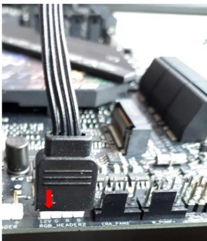
**CONNECTING THE D-RGB LED (LED with 3 wires)**
