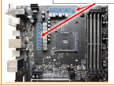
Replacement thermal pads @ EKWB web shop: Thermal PAD F 1mm - (120x12mm) [EAN: 3830046996732]
