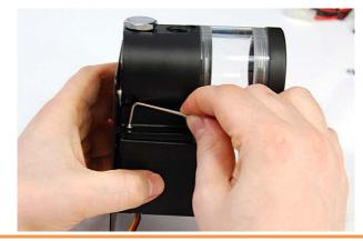
Cont.5: Use M3×6mm screws and M3 nut to attach the mounting bracket.
