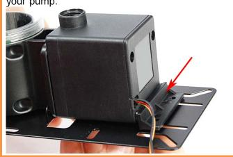
STEP 3: ATTACHING MOUNTING PLATE TO EK-RESERVOIR COMBO DCP 4.0
