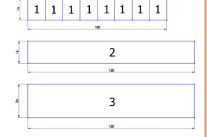
4. PLACING THERMAL PADS ON PCB. Place thermal pads on the circuit board as shown on the picture below. Refer to numbering in previous picture when applying thermal pads of different sizes or thicknesses. EK made sure to provide customers with more than adequate quantity of thermal pads to complete this step.
