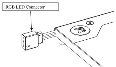
Plug the 4-pin connector from Water block's RGB LED light to the RGB\_HEADER on the motherboard. The LED will work if the pin layout on the header is as follows: **+12V G R B**.
