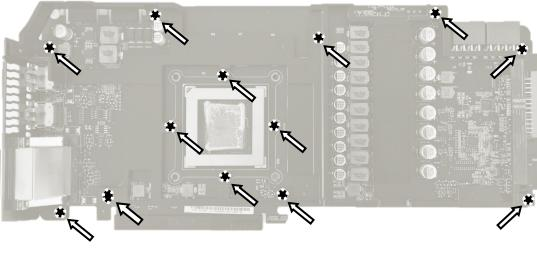
2. APPLYING THERMAL COMPOUND: Wipe off the remains (by using non-abrasive cloth or *q-tip*) of the original thermal compound until the components and circuit board are completely clean. Apply thermal compound: lightly coat NVIDIA GPU chip with enclosed EK-TIM Ectotherm thermal grease. EKWB recommends to apply thermal grease in cross form for best performance (see sample picture).
