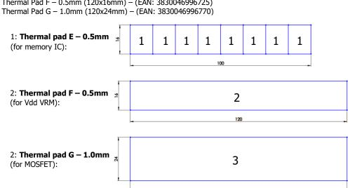
4. PLACING THERMAL PADS ON PCB. Place thermal pads on the circuit board as shown on the picture below. Refer to numbering in previous picture when applying thermal pads of different sizes or thicknesses. EK made sure to provide customers with more than adequate quantity of thermal pads to complete this step.
