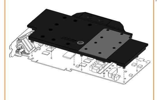
2. ATTACHING THE BLOCK TO THE GRAPHIC CARD. Use a Philips screwdriver screw with the enclosed M2,5x4 AX1 screws and one M2,5x6 AX1 screw. EKWB recommends users to start tightening the screws around the GPU core and continue outwards. <u>Always use</u> a plastic washer under each and every screw! If the washer is already present on the circuit board (usually around the four GPU core screw holes) there is no need for additional washer.
