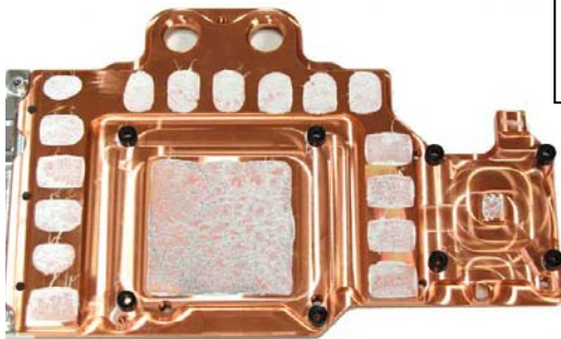
Picture 7: Placing/fixing the standoffs.
