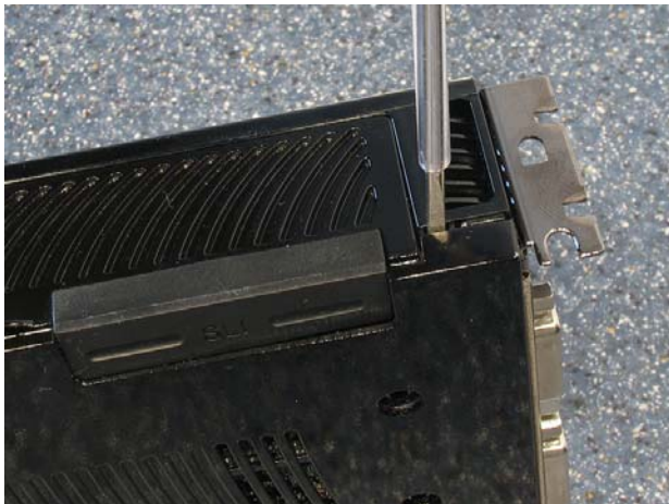
Picture 7: Disassembling the top part 5
