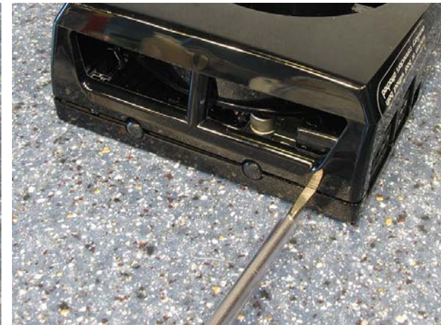
Picture 8: Disassembling the top part 6
