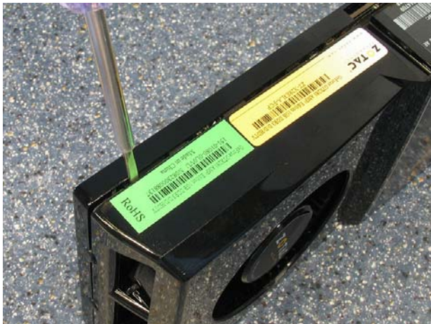
Picture 5: Disassembling the top part 3
