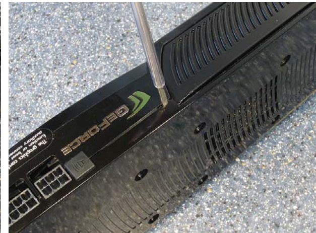
Picture 6: Disassembling the top part 4
