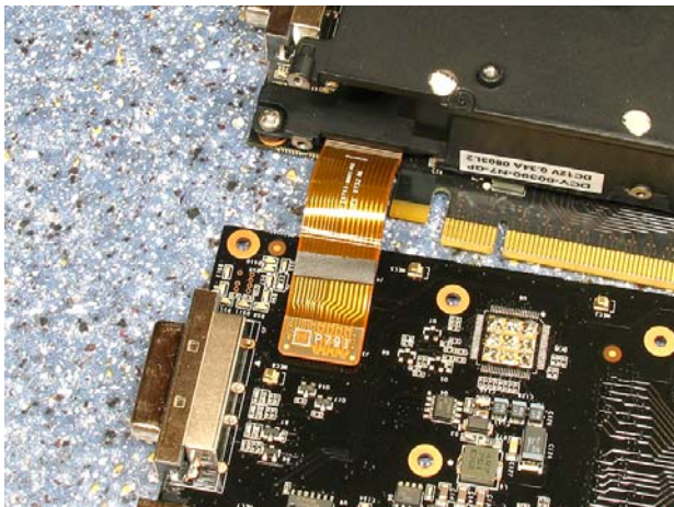
Picture 8: Disassembling - SLI bridge connection
