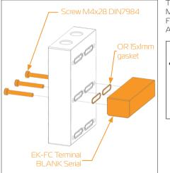
Tighten the three (3) enclosed M4x28 DIN7984 screws to EK-FC Terminal BLANK Serial using Allen (hex) key 2.5mm.
