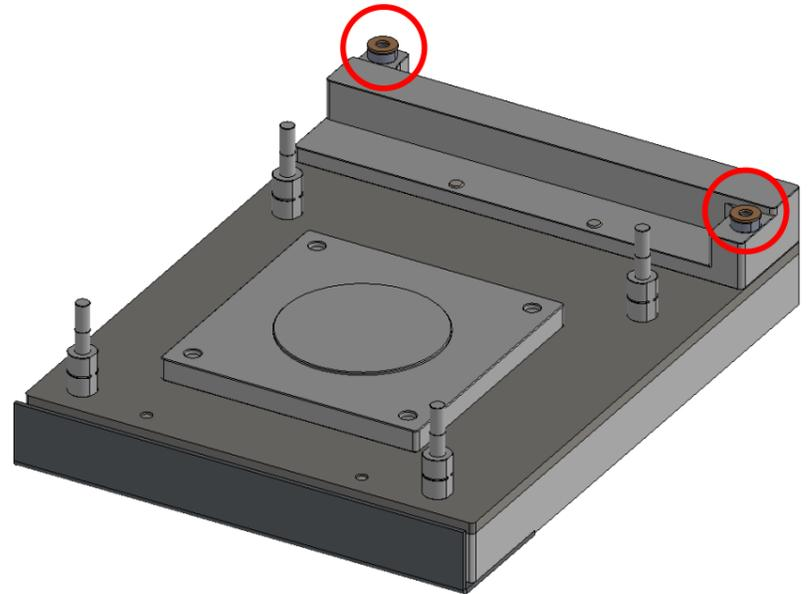
PLACING THE BLOCK ON THE MOTHERBOARD. Place the EK-FB MSI X299 GAMING PRO CARBON RGB Monoblock series water block gently to the motherboard or vice versa (as shown on photo below). Make sure that mounting holes are aligned.
