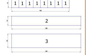
4. PLACING THERMAL PADS ON PCB. Place thermal pads on the circuit board as shown on the picture below. Refer to numbering in previous picture when applying thermal pads of different sizes or thicknesses. EK made sure to provide customers with more than adequate quantity of thermal pads to complete this step.
