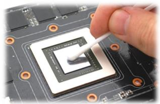
2. APPLYING THERMAL COMPOUND: Wipe off the remains (by using non–abrasive cloth or *q-tip*) of the original thermal compound until the components and circuit board are completely clean. Apply thermal compound: lightly coat *NVIDIA* GPU chip with enclosed EK-TIM Ectotherm thermal grease. EKWB recommends to apply thermal grease in cross form for best performance (see sample picture).
