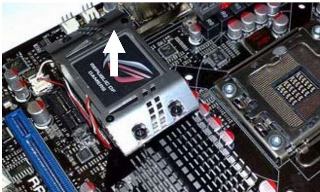
Picture 5: Also remove the level one small PCB plate (VTT CPU Power Card) under the small top box (republic of gamers logo)
