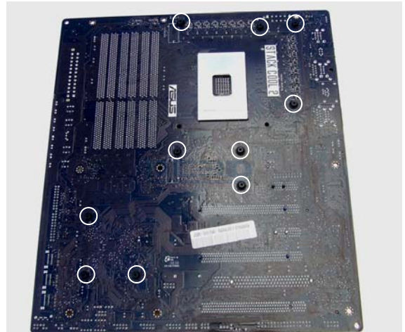
Picture 2: ASUS Rampage II Extreme motherboard – back (unscrew all 10 screws)
