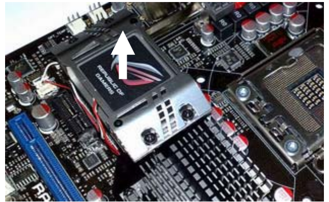
Picture 4: remove the small top box (republic of gamers logo) and unplug the connector
