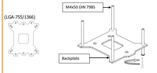
**3. Secure the backplate assembly** to the circuit board using M4 Nut, Metaland PVC washer. Continue with installation of the water block by following the STEP 2a!
