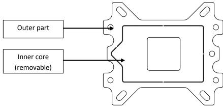
**2. Install the Backplate with pre-installed screws to the motherboard:** Make sure you use rubber gasket underneath the Backplate and mind the orientation of both metal as well as Backplate.
