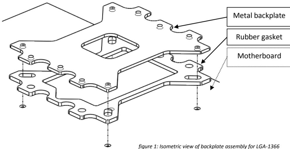
figure 1: Isometric view of backplate assembly for LGA-1366
