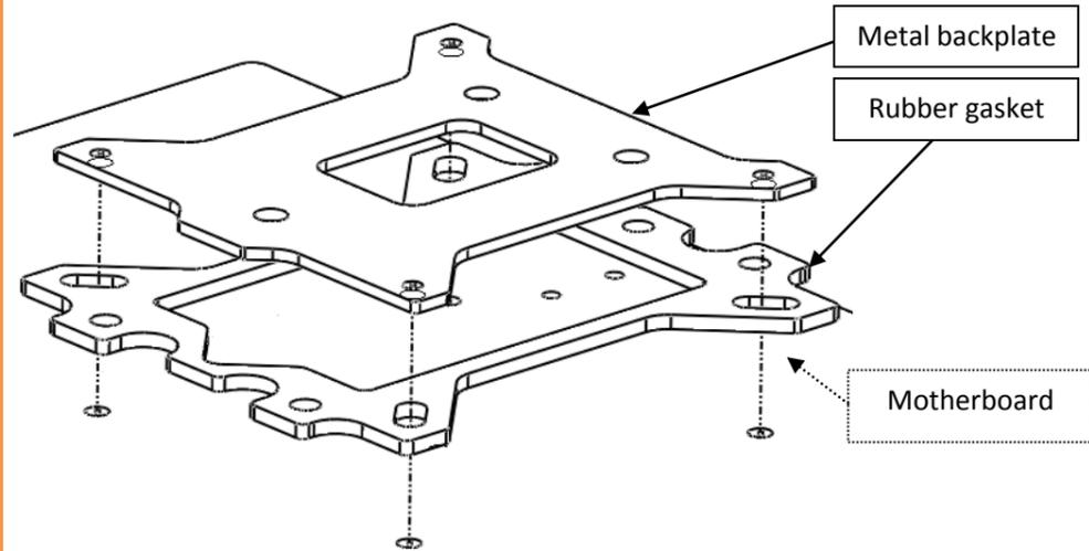
figure 2: Isometric view of backplate assembly for LGA-115x
