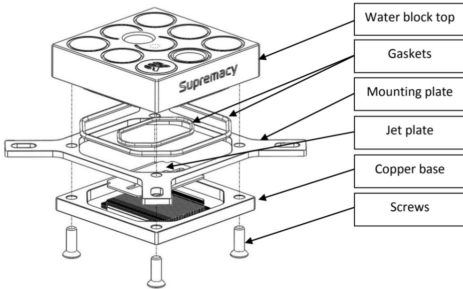
**Caution:** Narrow server type LGA-2011 is not supported by default – a **Mounting plate Supremacy LGA-2011 Narrow ILM** (EAN: 3830046990600) is mandatory to install this water block on narrow server type LGA-2011 motherboards.
