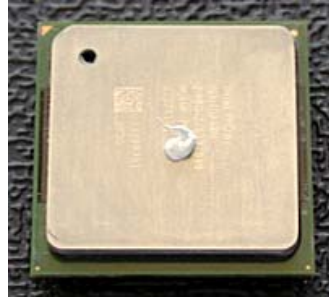
Picture 4: Applying compound on processor.
