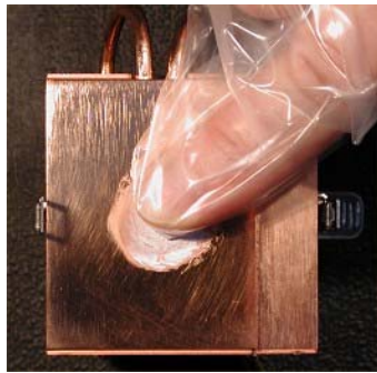
Picture 3: Applying compound on water block.
