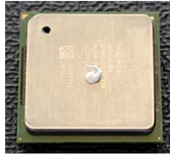
Picture 4: Applying compound on processor.
