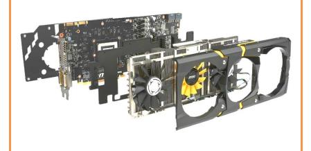
2. CLEANING THE PCB & APPLYING THERMAL COMPOUND. Carefully detach the original stock cooler after removing **all** screws securing it to the board. Wipe off the remains (by using non–abrasive cloth or *q-tip*) of the original thermal compound until the components and circuit board are completely clean. lightly coat *Nvidia* GPU chip with enclosed EK-TIM Ectotherm thermal grease. EKWB recommends to apply thermal grease in cross form for best performance (see sample picture).
