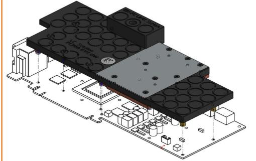
3. ATTACHING BLOCK TO THE GRAPHIC CARD. Use a Philips screwdriver screw in enclosed M3x4 DIN 7985 screws. EKWB recommends users to start tightening the screws around the GPU core and continue outwards. Always use a plastic washer under each and every screw!
