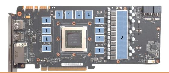
2. PLACING THE BLOCK TO THE GRAPHICS CARD. Carefully position the water block with preinstalled 2.5 mm standoffs on to the graphics card. During this process please make sure you align mounting holes on the PCB with holes on the water block. Also pay attention not to use too much force by pressing block down to PCB. Chip dies are prone to cracking.
