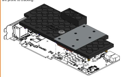
3. ATTACHING BLOCK TO THE GRAPHIC CARD. Use a Philips screwdriver screw in enclosed M3x4 DIN 7985 screws. EKWB recommends users to start tightening the screws around the GPU core and continue outwards.
