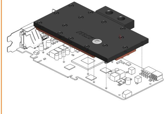
3. ATTACHING THE BLOCK TO THE GRAPHIC CARD. Use a Philips screwdriver screw with the enclosed M3x4 DIN 7985 screws. EKWB recommends users to start tightening the screws around the GPU core and continue outwards. <u>Always use</u> a plastic washer under each and every screw! If the washer is already present on the circuit board (usualy around the four GPU core screw holes) there is no need for additional washer.
