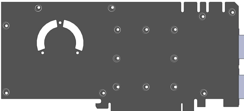
2. CLEANING THE PCB. Carefully detach the original heat sink after removing all fasteners securing it to the board and bracket. Wipe off the remains (by using non-abrasive cloth or Q-tip, as shown on sample photo) of the original thermal compound until the components and circuit board are completely clean. EKWB does not recommend using any liquids for removing paste.
