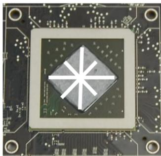
4. CUTTING THERMAL PADS. Your block comes with thermal pads, which have to be placed on chips (PLEASE REMOVE FOIL ON BOTH SIDES OF THERMAL PADS PRIOR TO INSTALLATION. WARNING: DIMENSION BELOW ARE SCALED.) All thermal pads are 1mm thick. Thermal pads #1 need to be cut to 4 pieces for RAM modules.
