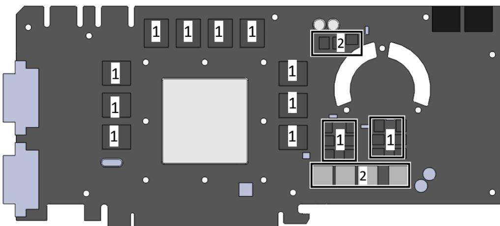
2. PLACING GPU REINFORCE PLATE ON PCB. Place metal reinforcer and reinforce washer on PCB as shown on picture below and screw it in with enclosed M3x4 screws. Make sure you use fasten screws equally and do not use too much force.
