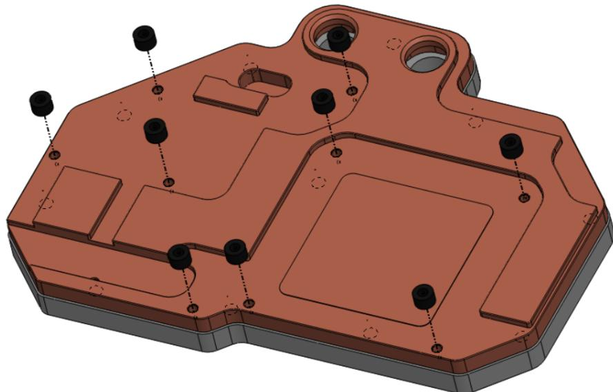
4. **ATTACHING BLOCK TO GRAPHIC CARD.** By using Philips screwdriver screw in enclosed M3x8 screws. EKWB recommends start screwing the screws around the GPU core and continue outwards.
