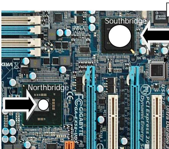
Picture 4: Apply thermal grease on NB and SB chipsets like shown in step 3. And 1mm thermal pad on Sata chip.
