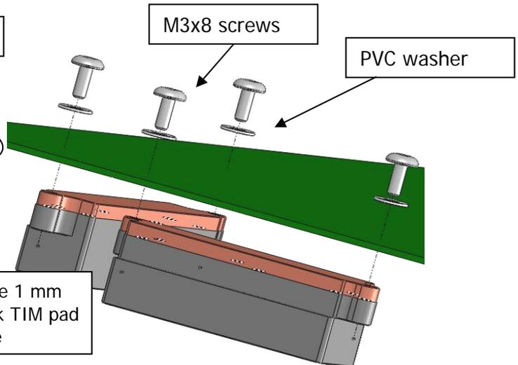
Picture 7: Installing 2 Mosfet blocks.
